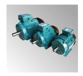
Motors are suitable for VFD operation, 5:1 ratio for constant torque applications, as higher grade and type of copper materials, lamination etc., are used and the motors undergo vacuum impregnated insulation treatment, thereby increasing the insulation strength on the overhangs of the motors so that harmonic distortions are minimized. Speed variations of 40 to 100% are recommended.
