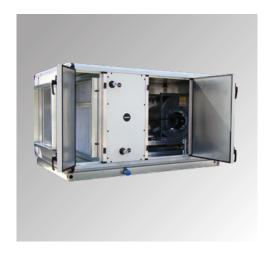
The outer surface of the panel is generally offered with pre-coated polyester, having excellent corrosion resistance, applied over galvanized steel sheet and further protected with vinyl guard film towards scratch protection. All plain galvanized steel sheets used shall have a minimum zinc coating of 270 GSM (G90) for anti corrosion.
