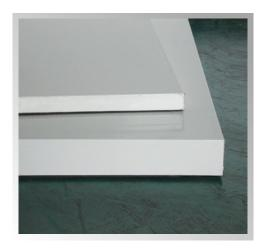
Polyol used for PUF insulation are blended with environment friendly CFC & HFC free agents, self extinguishable as per ASTM D 3014 standard and the foam insulation conforms to Class "O" of ISO 1182.2 standards. Thermal conductivity "K" factor is 0.02 W/m°K.
