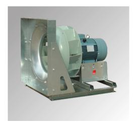
All the wheels are statically and dynamically balanced according to ISO 1940 and AMCA 204 – G2.5 standards. Clean room application fans with balancing grade of G1.0 can be provided upon request.
