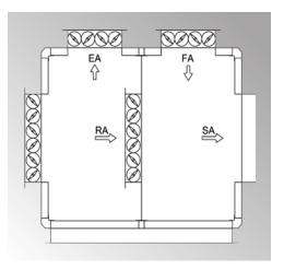
Inlet plenum sections are also offered to provide a proper means of air entry into the Air Handling Unit.
