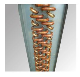
The cooler batteries are offered with a flexibility of choosing either ½"OD (12.5mm) or 5/8"OD (15.8mm) copper tubes depending on the capacities and water side pressure drops. Cooler batteries have an option of choosing water, glycol and refrigerants such as R22, R407C, R410a and R134a.
