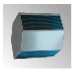
Plate type heat exchangers do not allow the passage of humidity from one flow to the other, but may use part of the latent heat contained in the humid exhaust air.
