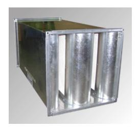
Sound attenuators are manufactured in square and rectangular sizes with round transitions to match the equipment internal dimensions. Attenuators are constructed out of 270 GSM zinc coated galvanized steel sheet to the standards of JIS 3302 / BS 2989 exterior sealed shell with sound absorbing baffles. The acoustic material is inorganic, incombustible, has a class 1 fire rating to BS 476 and non hygroscopic mineral fiber which is retained by means of galvanized perforated steel sheet.
