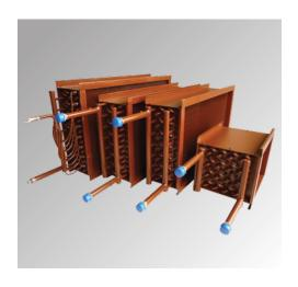
Coils are constructed out of corrugated aluminium fins and seamless copper tubes as standard. Anti corrosion coated coils or copper fins are provided upon request. The fins are of sine wave design and shall have collars drawn, belled and firmly bonded to the copper tubes by mechanical expansion of the tubes.
