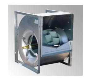
Wheels of forward curved fans are manufactured in galvanized steel construction, backward inclined and airfoil wheels in cold rolled steel sheet with polyester coated finish. Shafts are manufactured from C45 grade carbon steel and then coated for anti corrosion after assembly.
