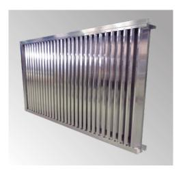
Cupro-nickel tubes and headers can be provided for special applications upon request where high acid or sand content tends to be corrosive or erosive. Each coil is factory pressure tested at 375 psig air pressure under water for water / steam coils and 450 psig for refrigerant coils for trouble free operations. Vent and drain plugs are provided for all water coils.
