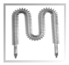
Heaters are available in 240V, 480V and 600V, 3 phase electrical characteristics. The heaters offer very negligible air side pressure drop ranging from 0.25Pa to 1.0Pa, depending on the air velocity and the number of rows of heating elements.
