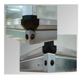
Base frames are made out of sendzimir galvanized steel sheets with either die cast aluminium joints or heavy duty steel joints with lifting holes. Hot dip galvanized channel frames are also provided, especially for larger dimension units.
